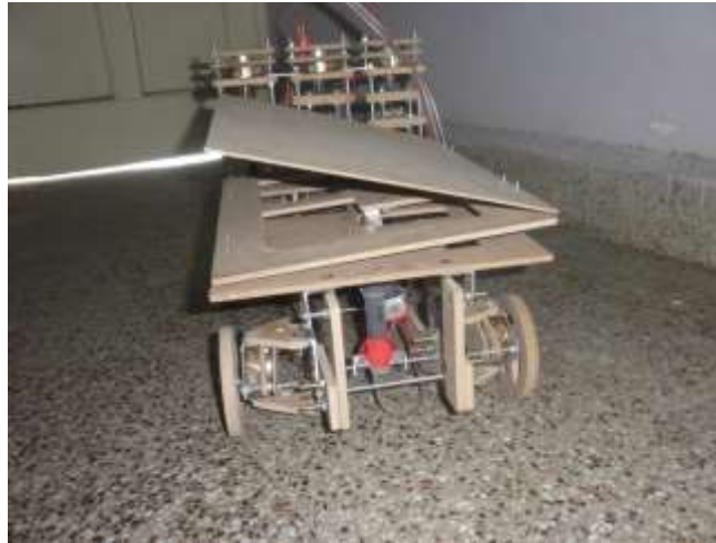
Fig.5.4: Right Side Dumping Action
